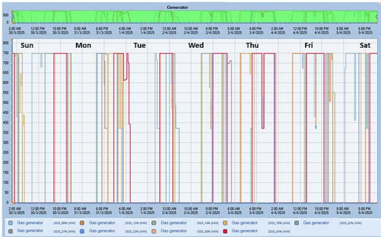
Figure 74 - Dispatch of a gas generator over a sample week
