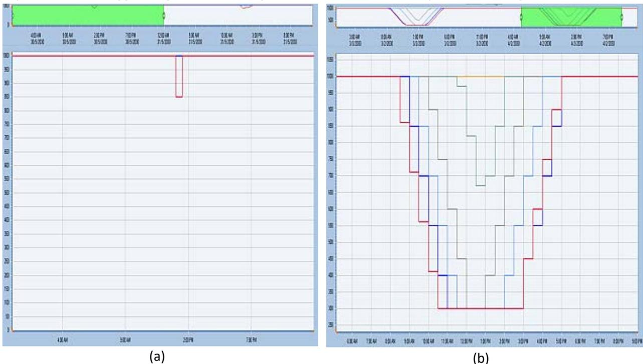
Figure 88 - Dispatch of a coal generator on (a) a high demand day and (b) a low demand day
