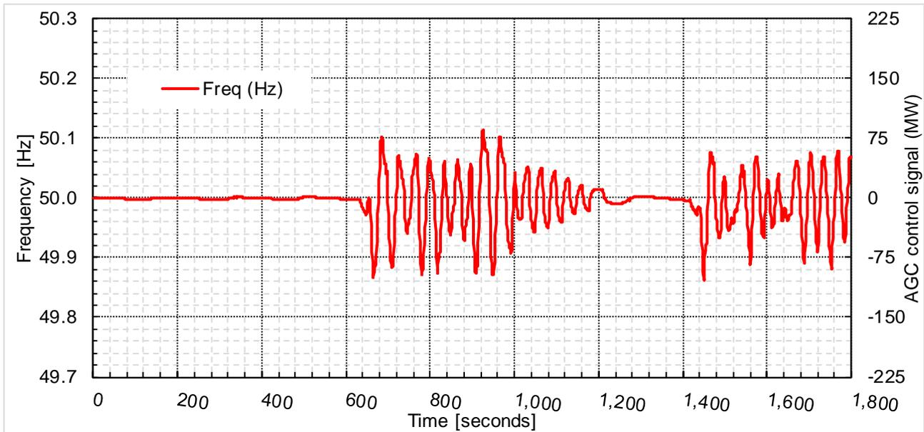
Figure 117 – System frequency response for the 30-min AGC testing window
