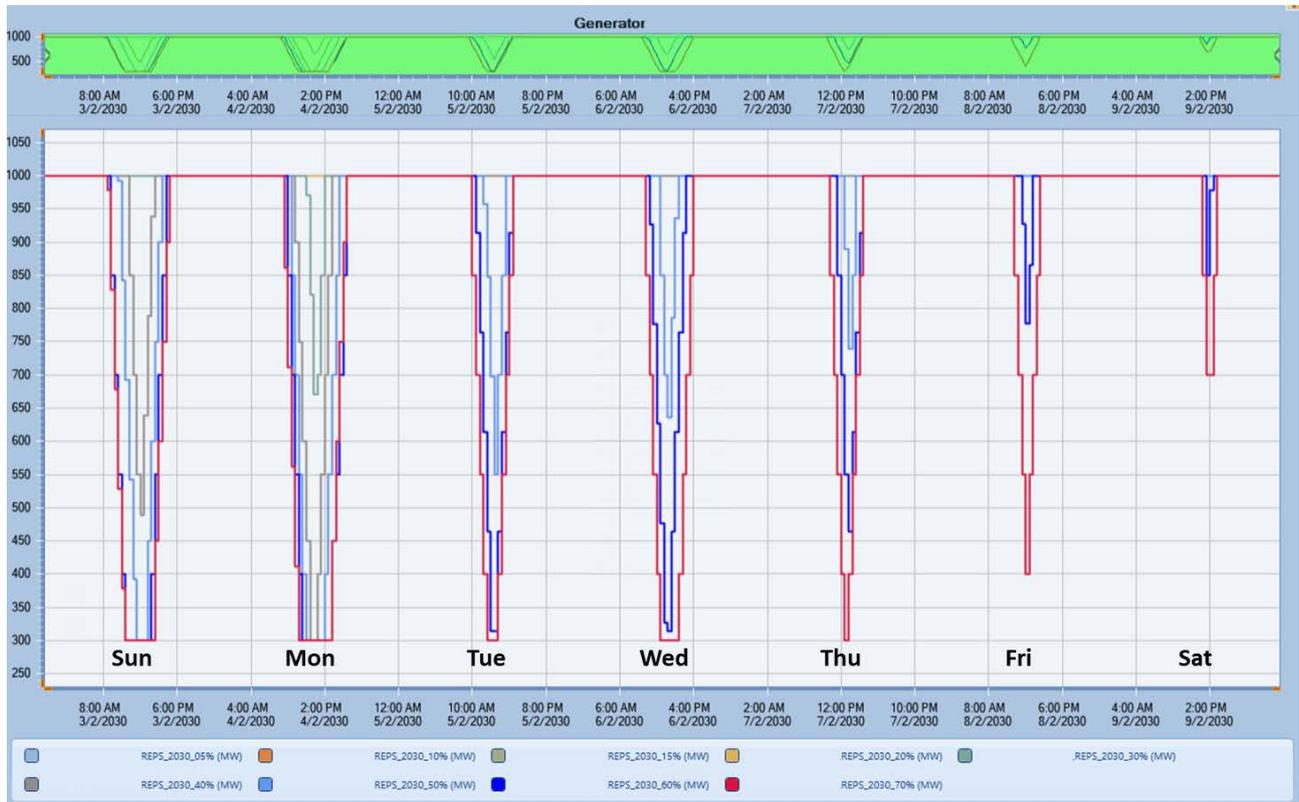
Figure 87 - Dispatch of a coal generator over a sample week
