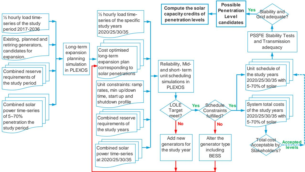
Figure 44 – Long-term capacity planning, mid/short-term operation and grid study workflow
