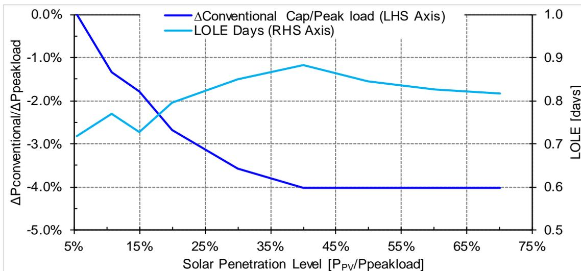
**Figure 56 – Reduction of conventional capacity and LOLE vs penetration level 2030**
