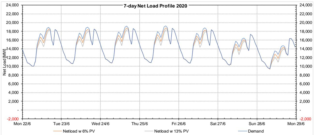
Figure 59 - Netload profile of a normal week in 2020 with tested penetration levels
