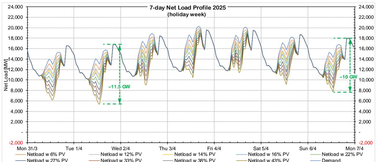
Figure 68 - Netload profile of a holiday week in 2025 with tested penetration levels
