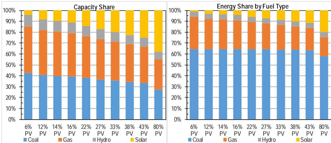
Figure 71 – Capacity and energy share for year 2025 without gas constraint
