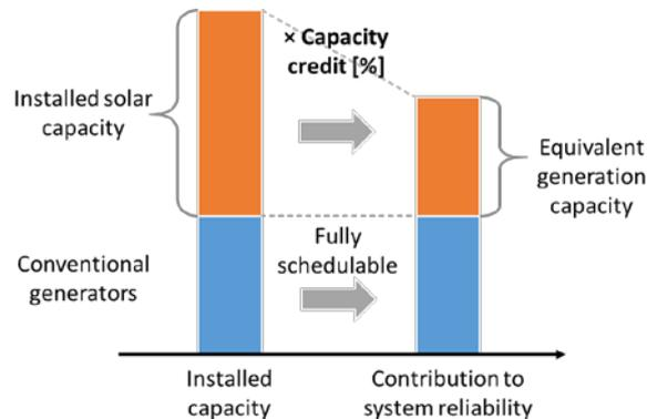
**Figure 123 – Equivalent capacity of solar generation**
