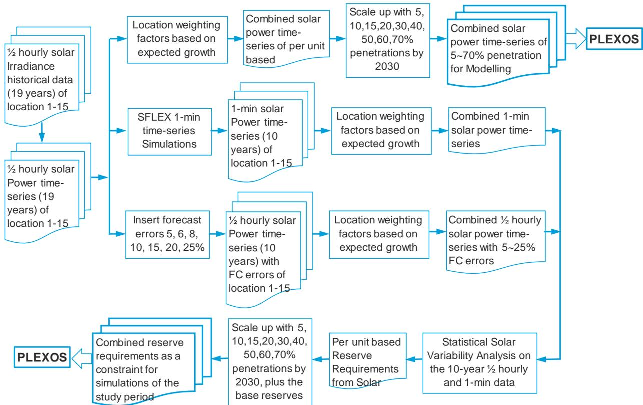
Figure 43 – Data processing and solar variability analysis workflow
