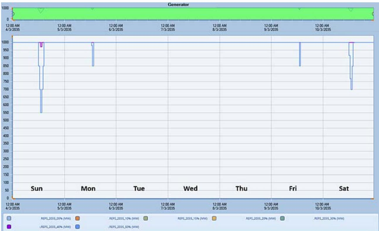
Figure 99 - Dispatch of a coal generator over a sample week 5-50% penetration in 2035
