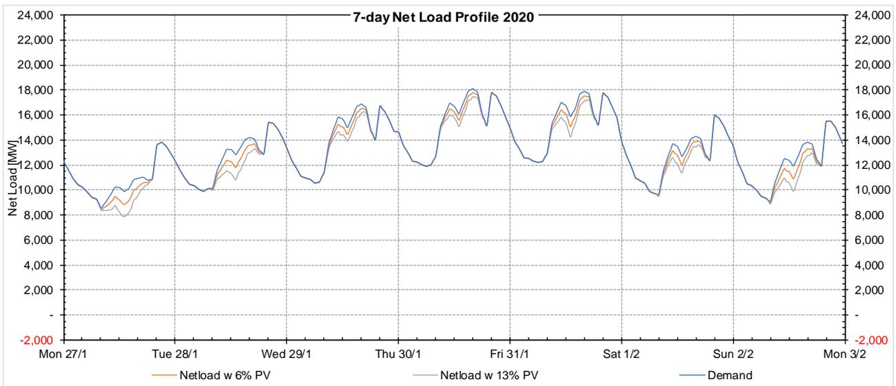
Figure 60 - Netload profile of a holiday week in 2020 with tested penetration levels
