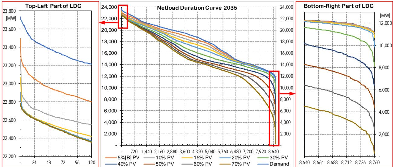
Figure 95 - Netload duration curves with tested penetration rates in 2035
