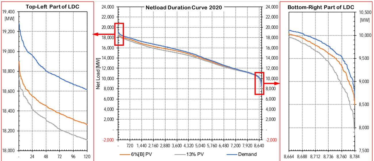
Figure 61 - Netload duration curve for 2020
