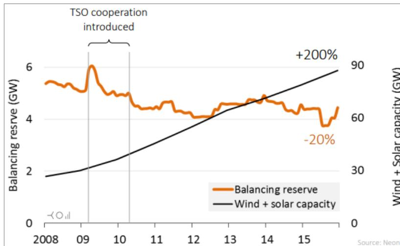
Figure 27 – Managed balancing reserve volume with increasing VRE penetration
