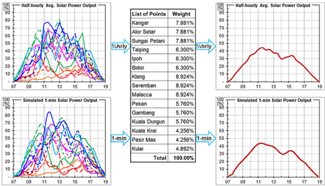
Figure 50 - Combining the power time-series with location weightage
