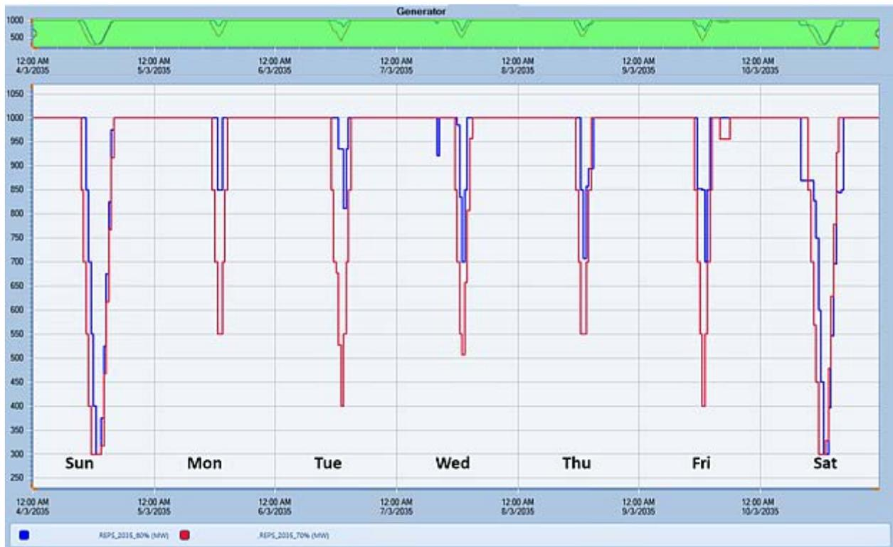
Figure 98 - Dispatch of a coal generator over a sample week with 60% and 70% solar in 2035
