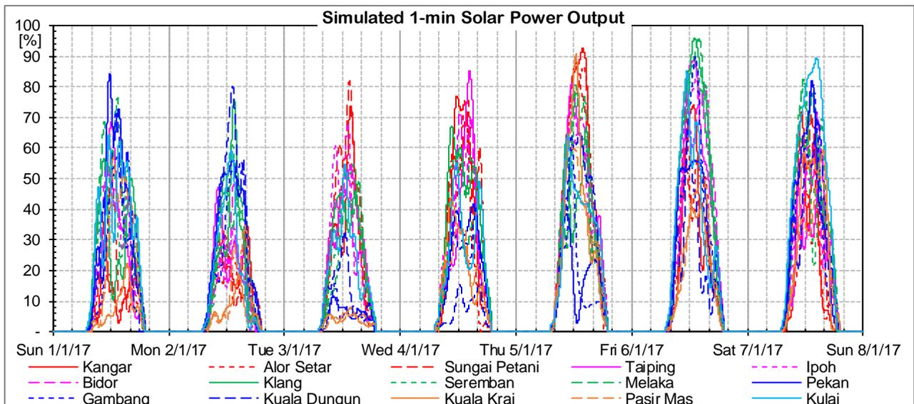
Figure 49 - Simulated 1-min solar power output for the sampled week
