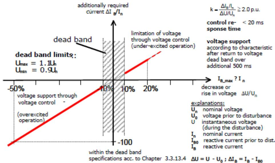
Figure 125 – German grid code requirement for voltage support from renewable generators
