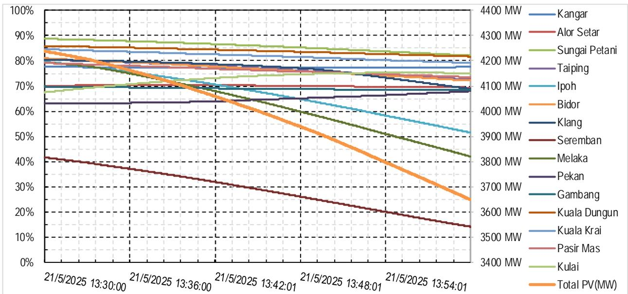
**Figure 116 – Individual and total solar generation fluctuation for AGC testing window**
