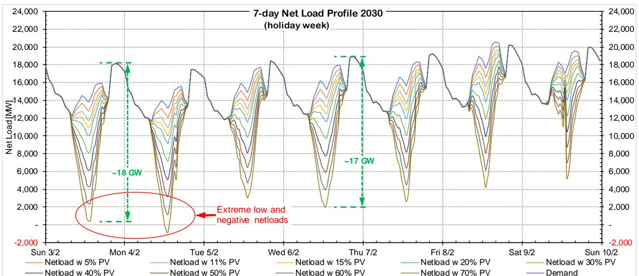
Figure 83 - Netload profiles of a holiday week in 2030 with tested penetration levels
