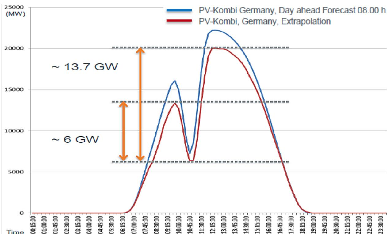
Figure 23 – Short time high magnitude fluctuation due to solar eclipse
