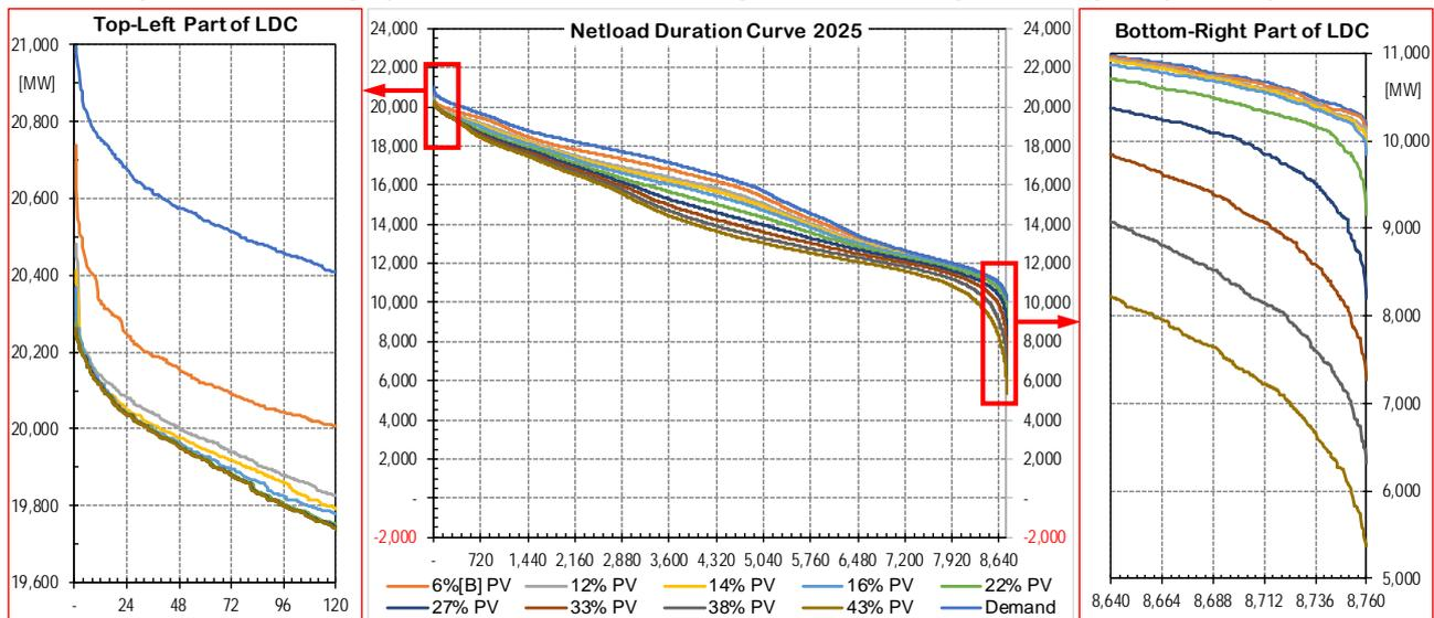
Figure 69 - Netload duration curves for year 2025 with tested penetration levels
