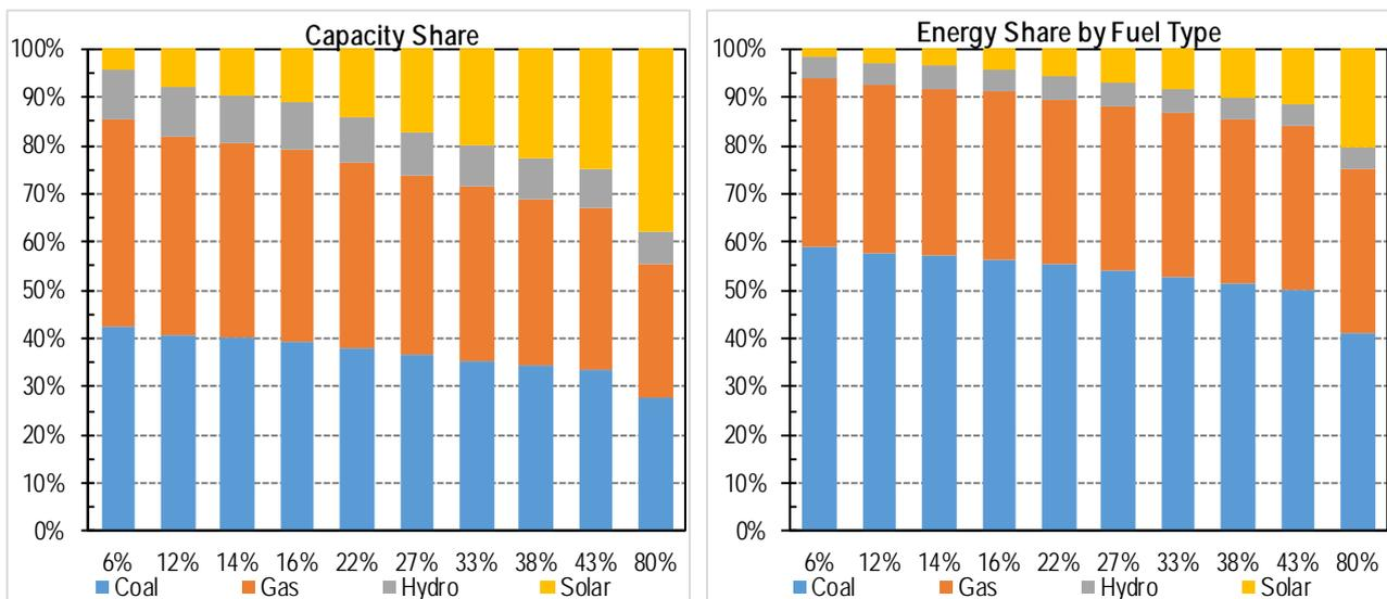
Figure 77 – Capacity and energy share for year 2025 with gas constraint
