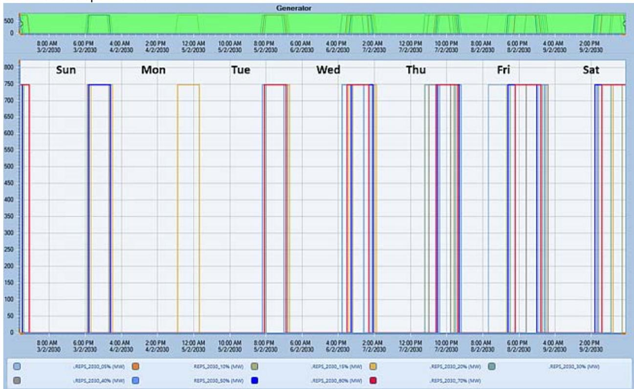
Figure 89 - Dispatch of a gas generator over a sample week
