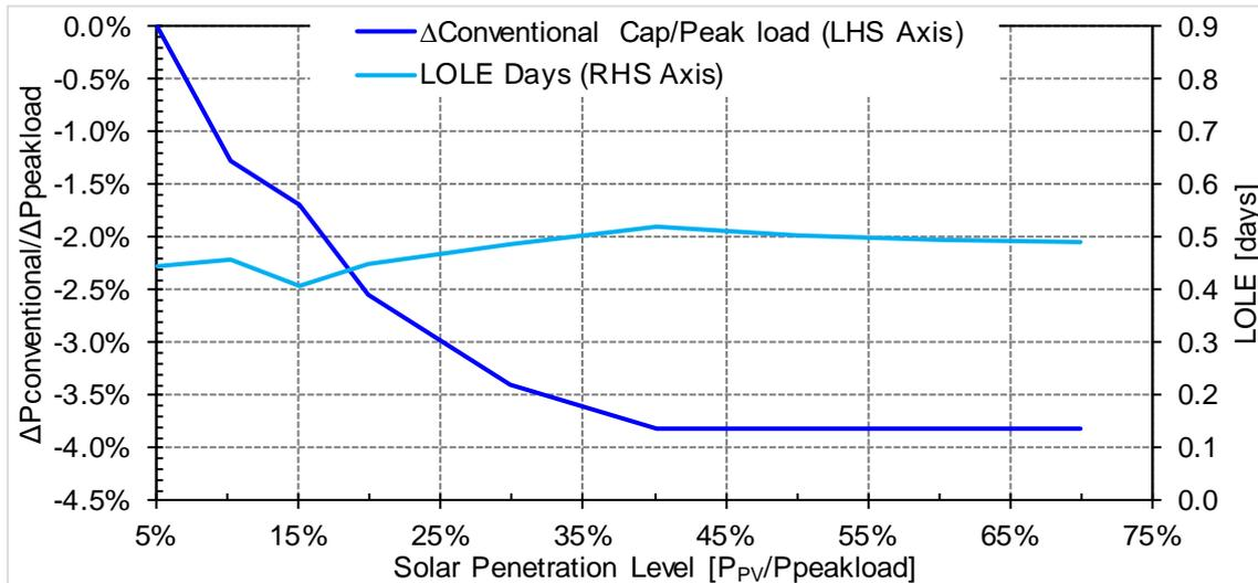
Figure 57 – Reduction of conventional capacity and LOLE vs penetration level 2035
