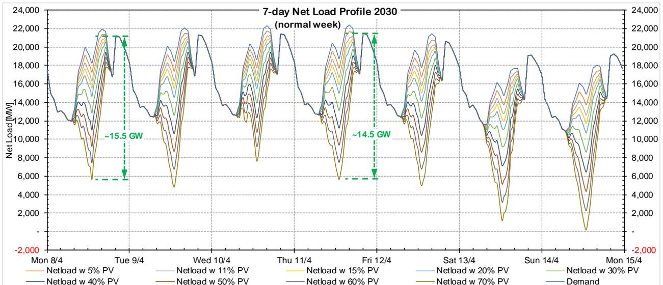
Figure 82 - Netload profiles of a normal week in 2030 with tested penetration levels
