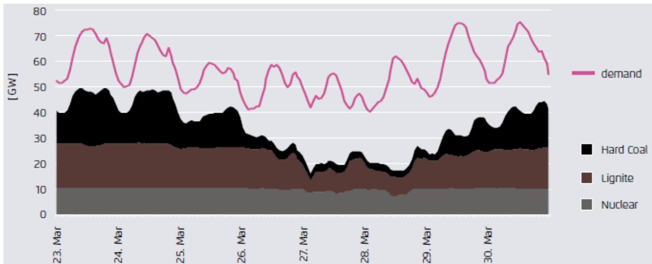
Figure 28 – Flexible operation of conventional generators
