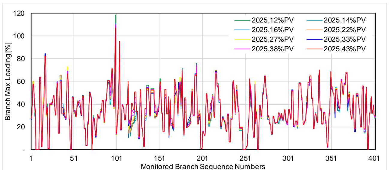
Figure 109 - Branch maximum loadings under different PV penetration levels
