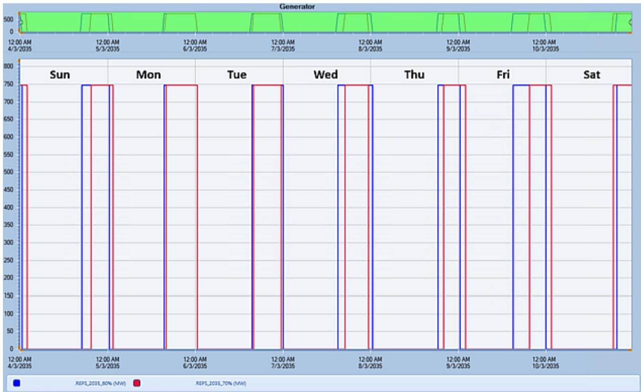
Figure 102 - Dispatch of a gas generator over a sample week with 60-70% PV generation
