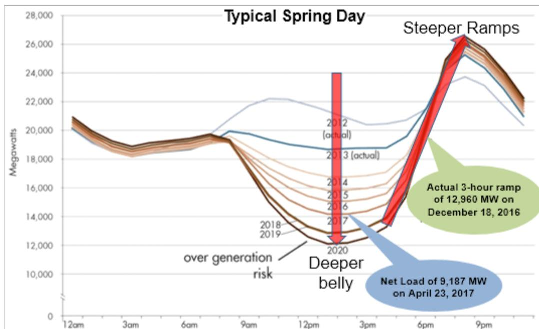
Figure 31 – California grid net-load profile of typical spring day
