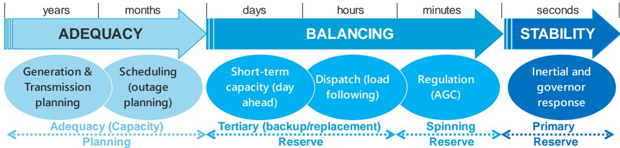
Figure 39 – Aspects of a grid system planning and operations
