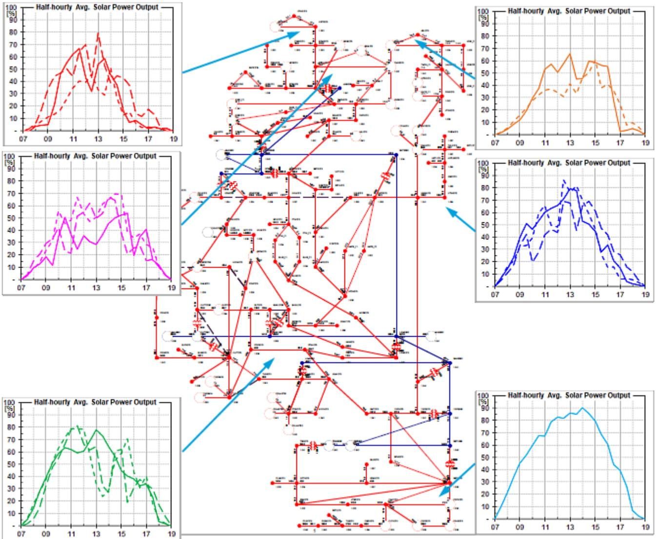
Figure 106 - Grid transmission backbone and PV connection points
