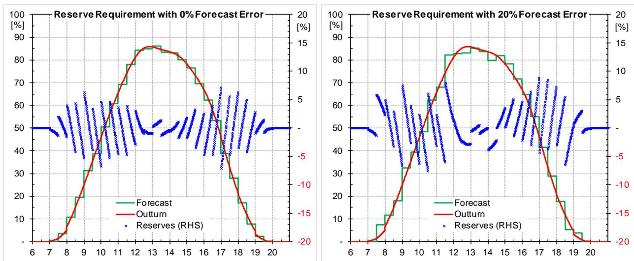
**Figure 53 – Delta power within a dispatch interval with 0% and 20% forecast error**
