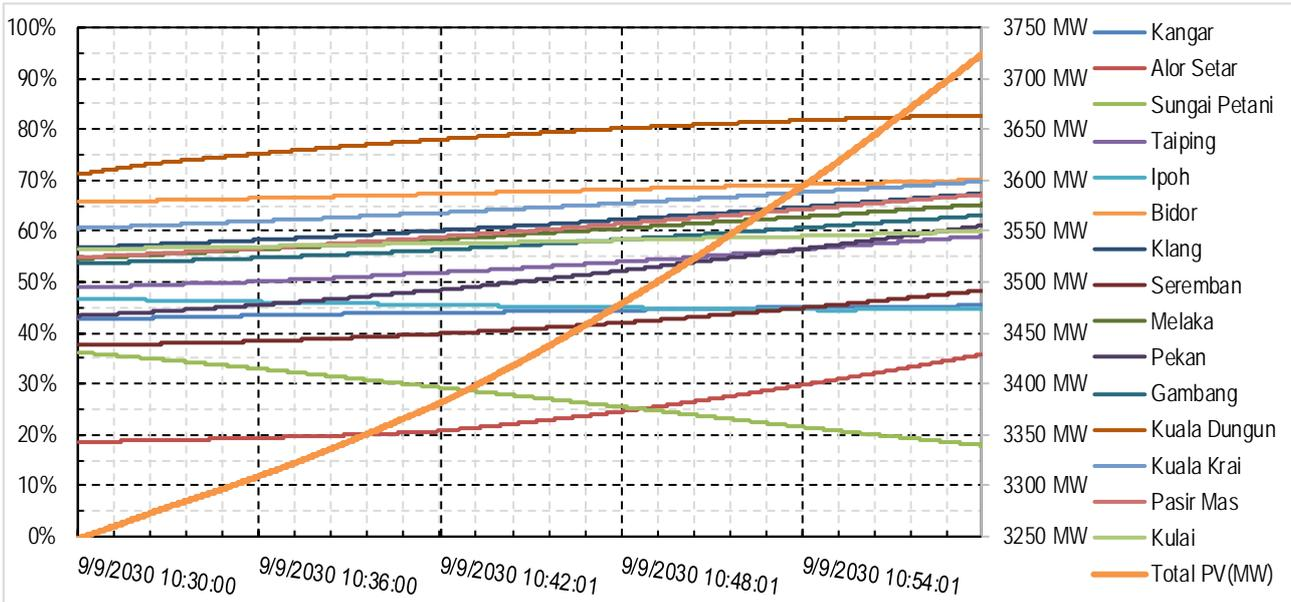
Figure 121 – Individual and total solar generation fluctuation in 30-min AGC testing window
