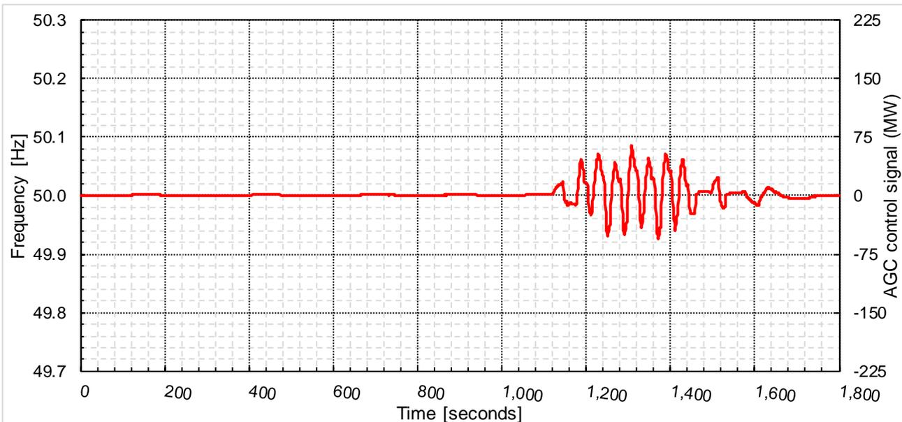
Figure 122 – System frequency profile in the 30-min AGC testing window
