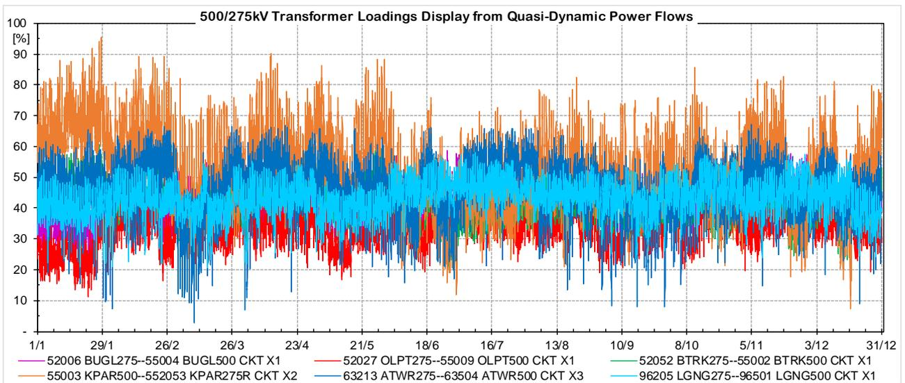
Figure 108 - Full year loading of selected 500/275kV inter-bus transformers
