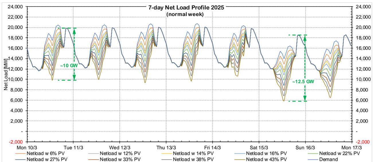
Figure 67 – Netload profile of a normal week in 2025 with tested penetration levels
