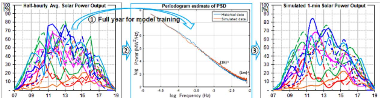
Figure 47 – Half-hourly to 1-min data simulation
