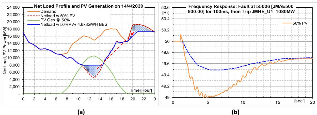
**Figure 126 Illustrative BES Applications: (a) netload profile conditioning, (b) inertia response**
