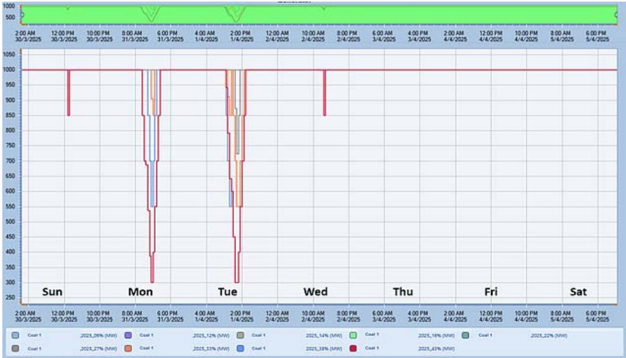
Figure 72 - Dispatch of a coal generator over a sample week
