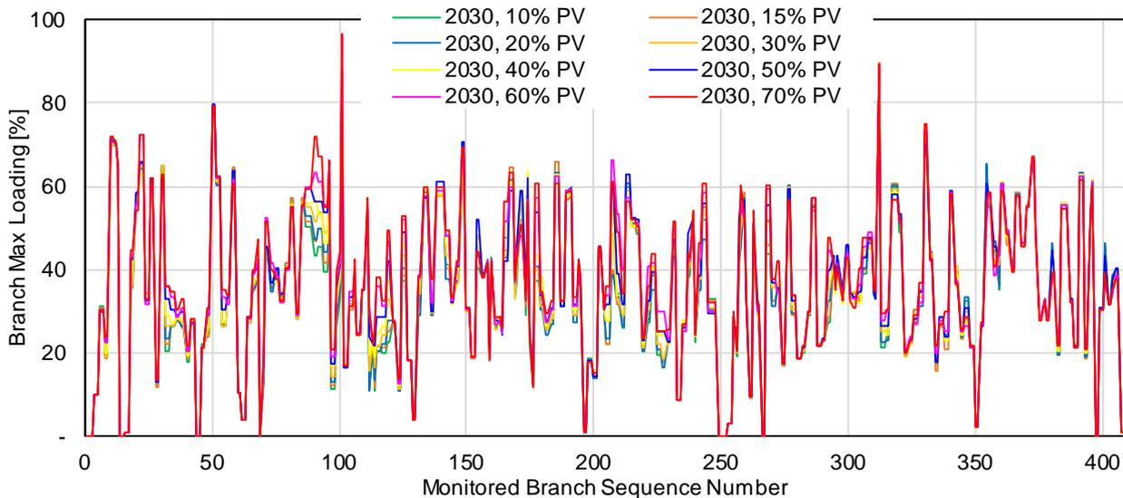
Figure 110 – Backbone bus maximum loading percentage under different PV penetration rates
