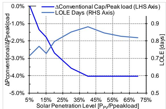
Figure 129 – Summary: Capacity planning for solar penetration levels
