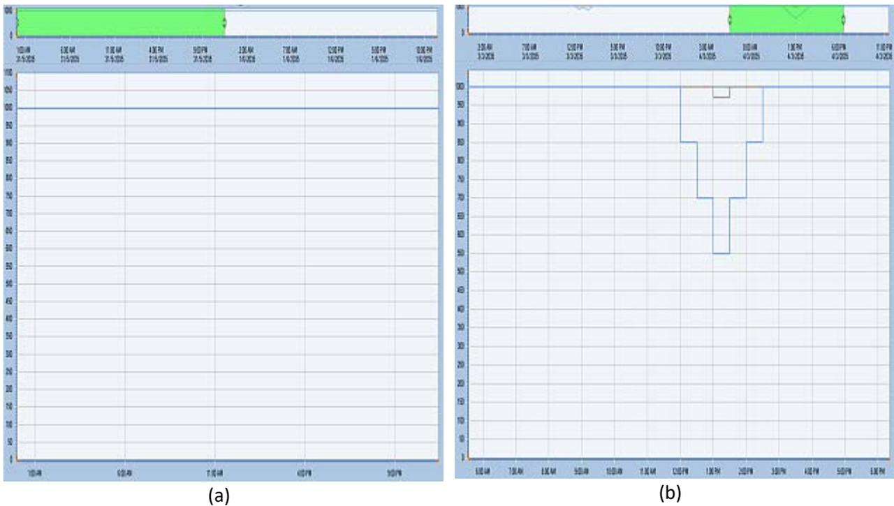
Figure 101 - Dispatch of a coal generator with 5-50% PV penetration on (a) a high demand day and (b) a low demand day
