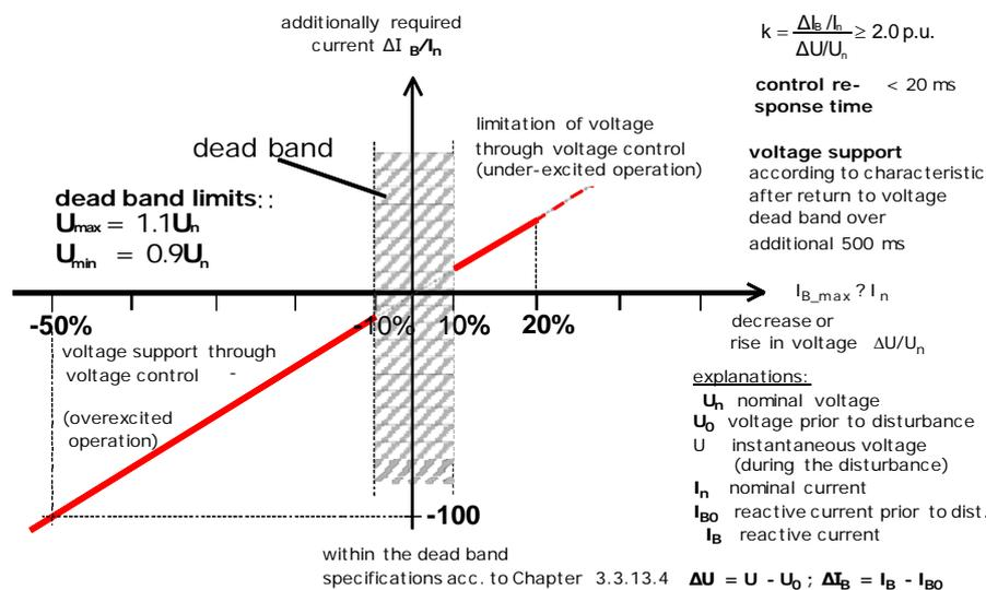
Figure 138 – German grid code requirement for voltage support from renewable generators
