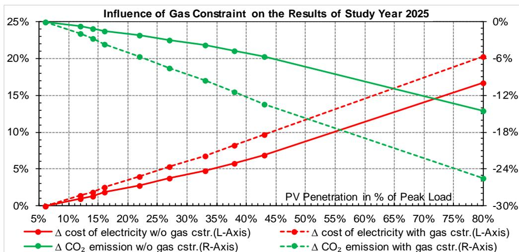
Figure 78 – Comparison of results with and without gas constraint
