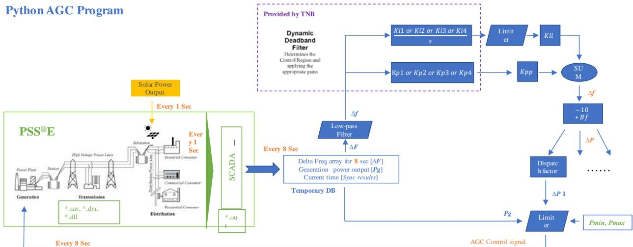
**Figure 115 – AGC test setup with PSS®E in Python**
