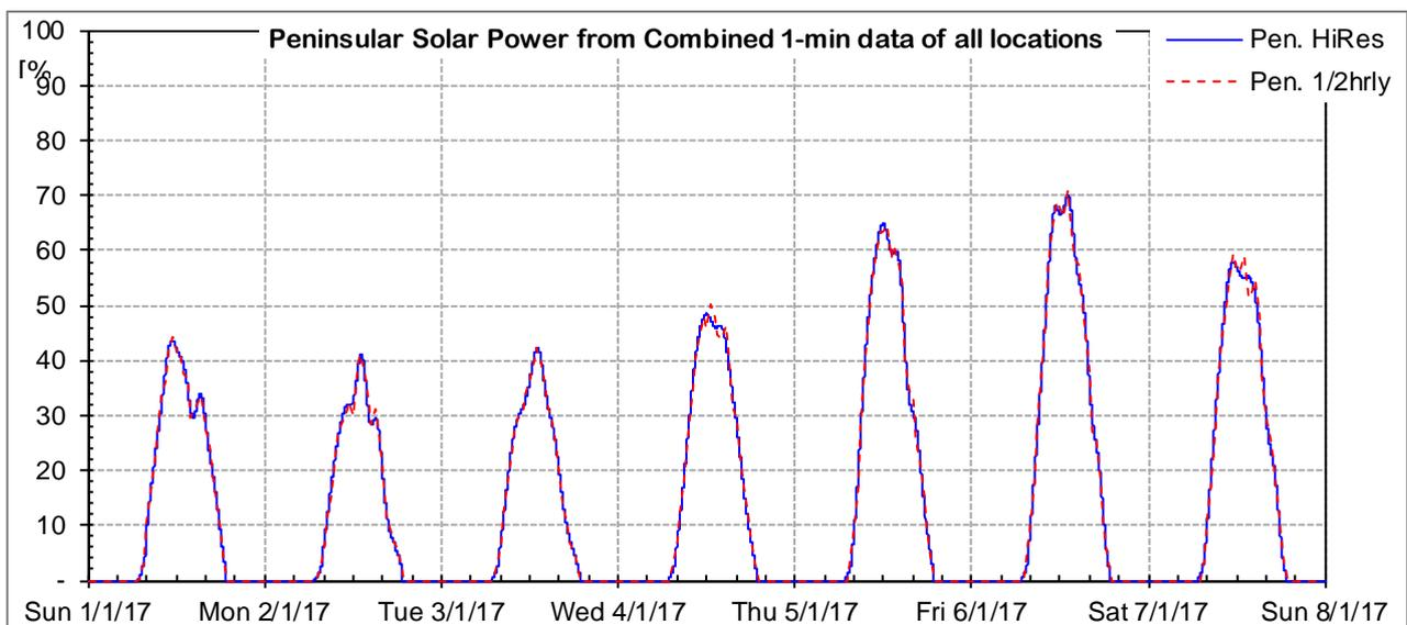
Figure 51 - Combined half-hour and 1-min solar power output for the sampled week
