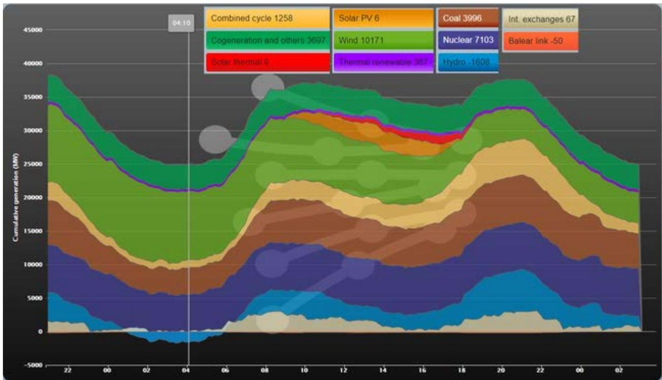
Figure 38 – Resulted generation mix due to mismatch of load and wind generation profiles <sup>64</sup>
