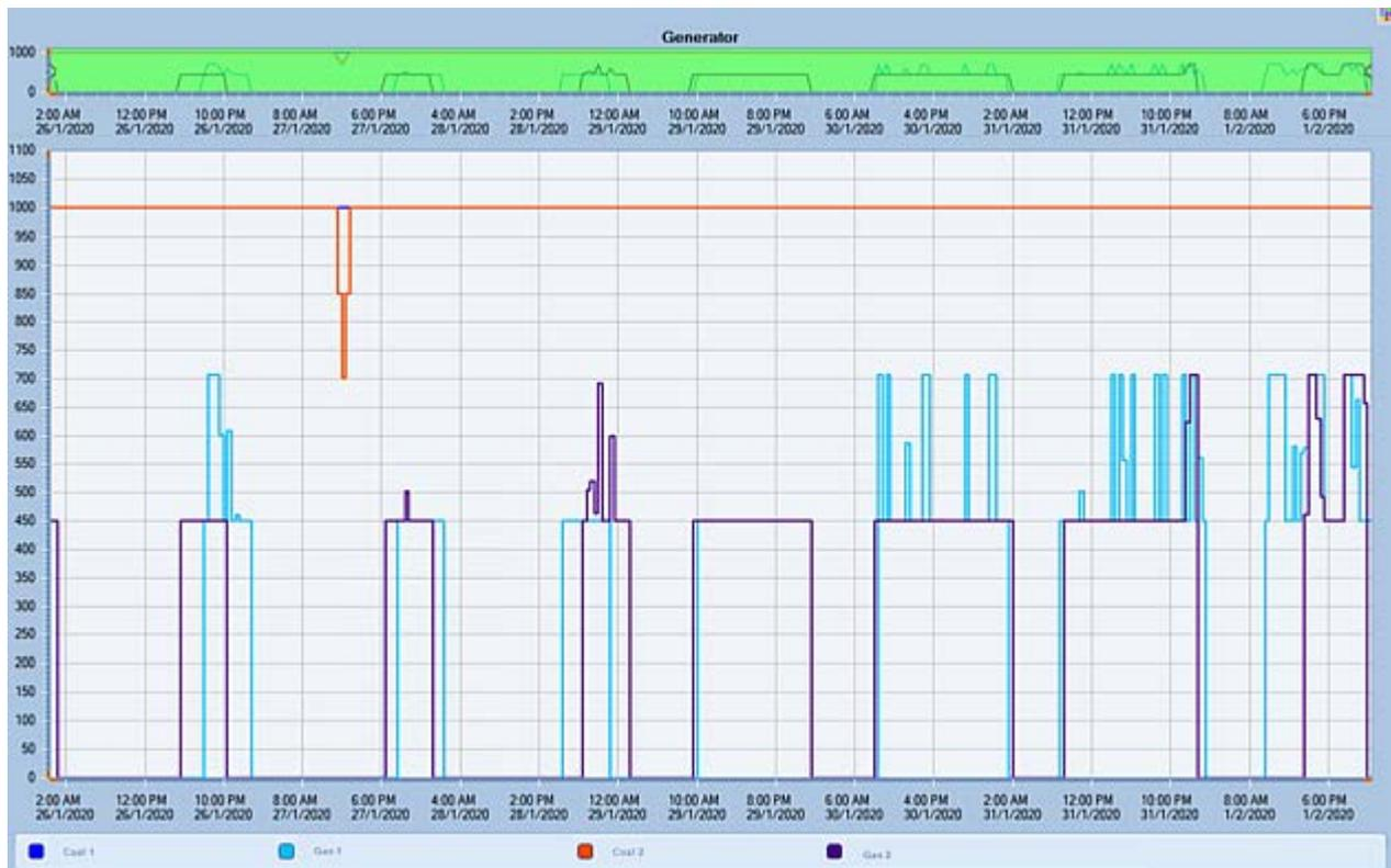
Figure 63 – Dispatch of gas and coal generators on a low demand day
